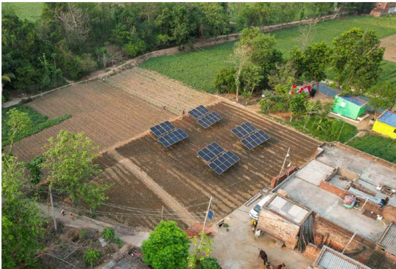
In Bihar's Gaya district, TCI built a 20-kW agrivoltaics installation for a group of six farmers. (Photo by TCI)
